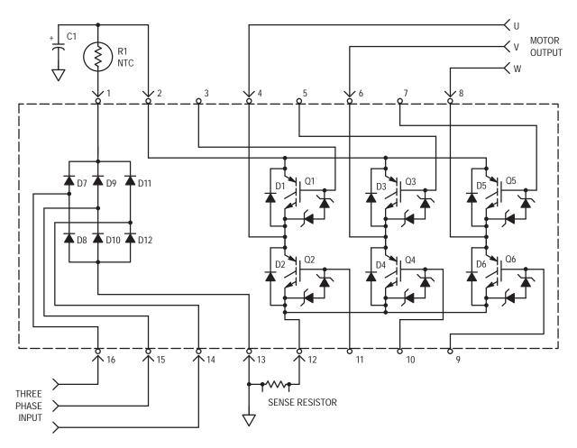
Figure 10–1. 16 Pin VersaPower™ Three Phase Input and 6–Pack
