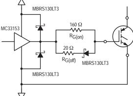
Figure 5. Recommended Gate Drive Circuit
