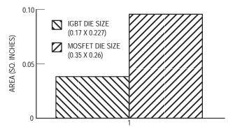
Figure 1–1b. Reduced Die Size of IGBT Realized When Compared to a MOSFET with Similar Ratings
