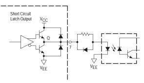
A negative bias voltage can be used to drive the IGBT into the off-state. This is a practice carried over from bipolar Darlington drives and is generally not required for IGBTs. However, a negative bias will reduce the possibility of shoot-through. The MC33153 has separate pins for V<sub>EE</sub> and Kelvin Ground. This permits operation using a +15/-5.0 V supply.
