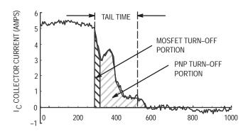
Figure 1–5. IGBT Current Turn–off Waveform
