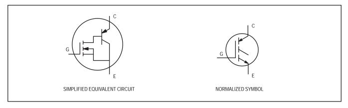
Figure 12–5. Basic standard IGBT equivalent circuit
