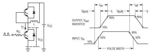
Figure 19. Inductive Switching Time Test Circuit and Timing Chart
