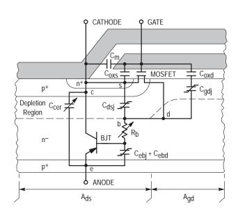
Figure 5–5. IGBT Equivalent Circuit Superimposed on One–half of Symmetric IGBT Cell (Reprinted with permission from NIST)
