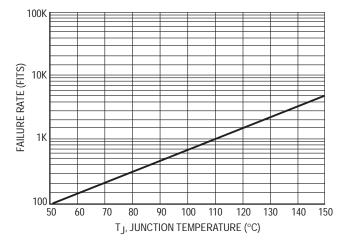
Figure 16–2. High Temperature Gate Bias Failure Rate versus Junction Temperature
