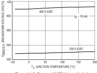
Figure 11–5. Clamped IGBT Voltage Variation Over Temperature
