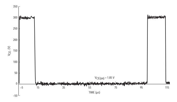
Figure 8–7. Typical  $V_{CE}$  Waveform of the Motorola Generation 2 IGBT in a 1 HP Motor Drive at 1750 RPM
