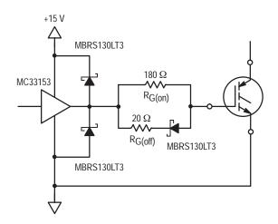
Figure 5. Recommended Gate Drive Circuit
