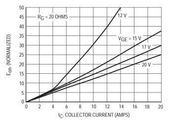
Figure 4–1. Turn–on Loss with Different Gate–Emitter Voltage
