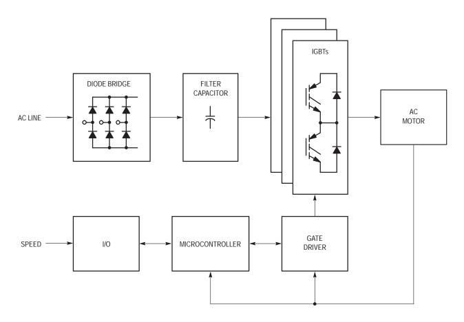
Figure 7–2. Typical IGBT AC Motor Drive Application
