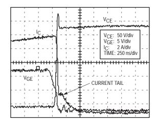
Figure 5–4a. Turn–off Waveforms at 25°C
