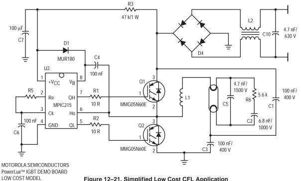
Figure 12–21. Simplified Low Cost CFL Application
