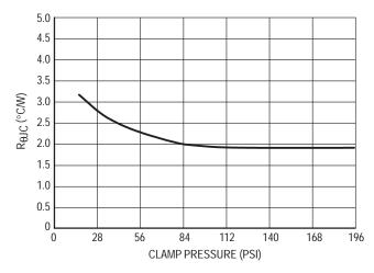
Figure 15–4. R<sub>0</sub>JC versus Clamp Pressure
