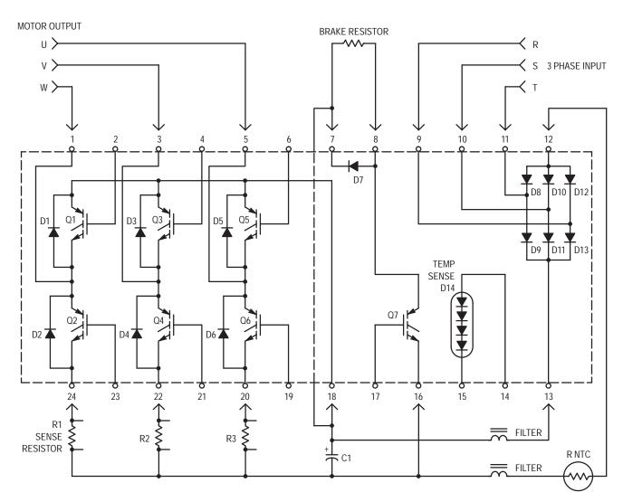
Figure 8. Schematic of Module, Showing Pin–Out and External Connections
