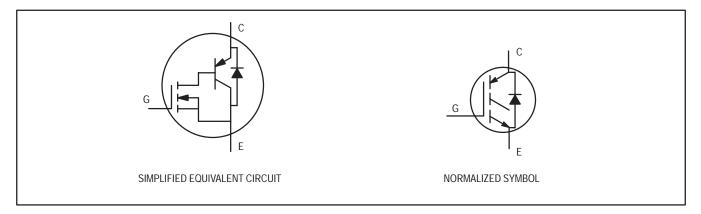
Figure 12–10. Simplified IGBT Equivalent Circuit
