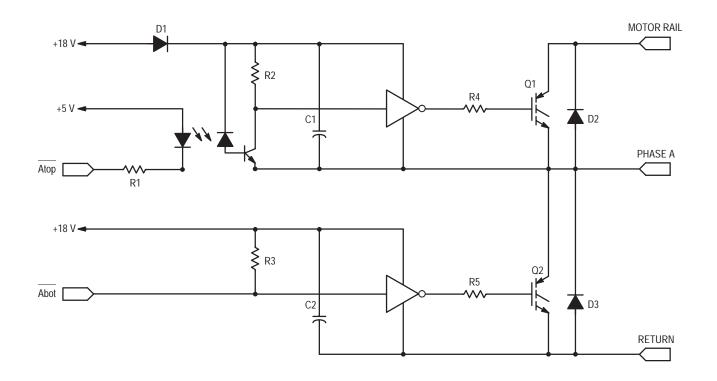
Figure 13–1. Minimal N–Channel IGBT Power Stage
