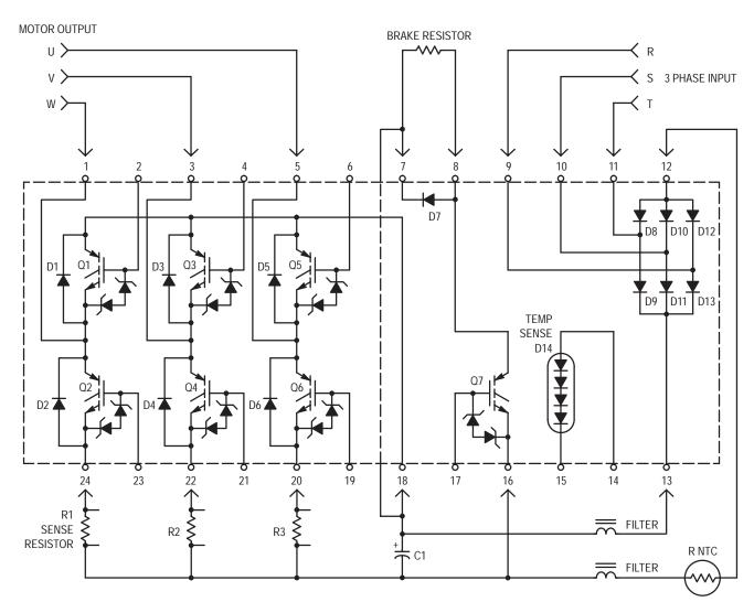
Figure 9. Schematic of Module, Showing Pin–Out and External Connections
