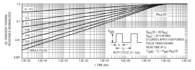
Figure 12. Typical Thermal Response
