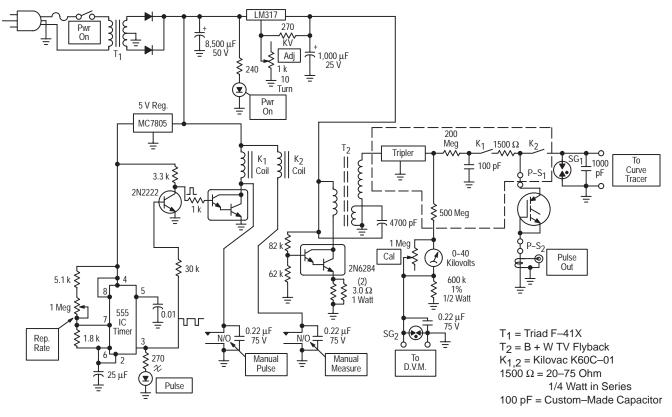
Figure 17–3. ESD (Electrostatic Discharge) Tester with 40 Kilovolt Capability
