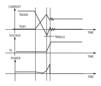
Figure 1–7. Waveforms Associated with Anti–Parallel Diode Turn–off
