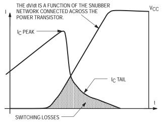
Figure 12-8. Switching Losses
