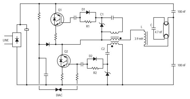
Figure 12-22. Self Oscillant, Low Cost CFL Basic Circuit
