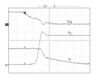
Figure 7–4a. IGBT Turn–Off Test Waveforms of STD Series MGW20N60D (100 ns/div) @ I<sub>C</sub> = 20 A, V<sub>CC</sub> = 360 V, V<sub>G</sub>/R<sub>G</sub> = 15 V/20 Ω, T<sub>J</sub> = 125°C
