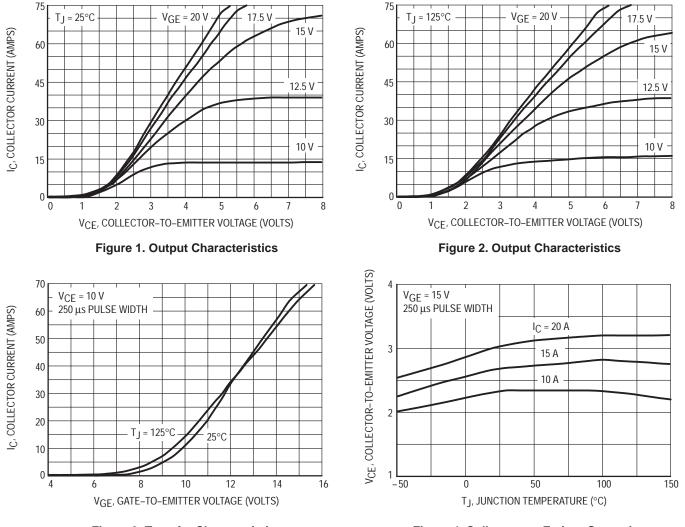
Figure 3. Transfer Characteristics
