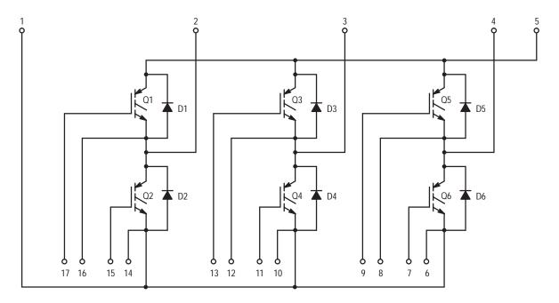
Figure 18. Schematic of Module, Showing Pin–Out
