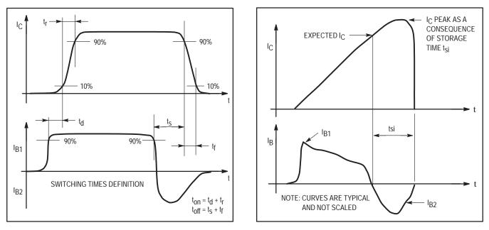
For a standard bipolar transistor, the storage time is dependent on the gain ( $\beta$ ) of the transistor associated with the operating point I<sub>C</sub> and the drive conditions I<sub>B1</sub> and I<sub>B2</sub>. The H2BIP device is free from this relationship, for a given I<sub>C</sub> range, and provides a far better design than older bipolar technology.
