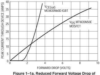
Figure 1–1a. Reduced Forward Voltage Drop of IGBT Realized When Compared to a MOSFET with Similar Ratings
