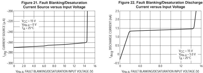
V<sub>CC</sub> = 15 V VPin 4 = 5.0 V  $T_A = 25^{\circ}C$ 8.0 16
