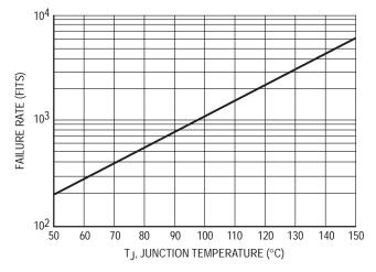
Figure 16–1. High Temperature Reverse Bias Failure Rate versus Junction Temperature
