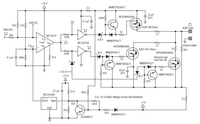
Figure 9–4. Gate Driver Circuit for Either Upper or Lower IGBT Power Devices
