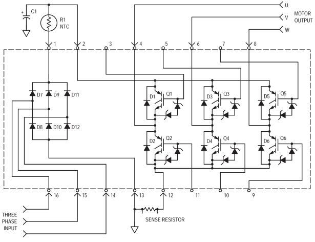
Figure 1. Schematic of Module, Showing Pin–Out and External Connections
