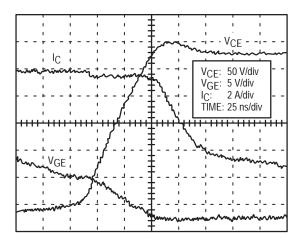
Figure 5–8. Turn–off at 120°C (V<sub>DD</sub> = 300 Vdc)
