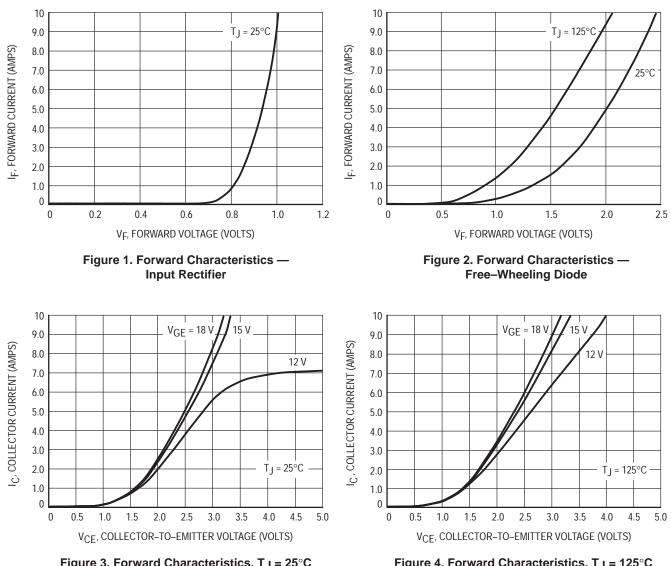
Figure 3. Forward Characteristics, T<sub>J</sub> = 25°C
