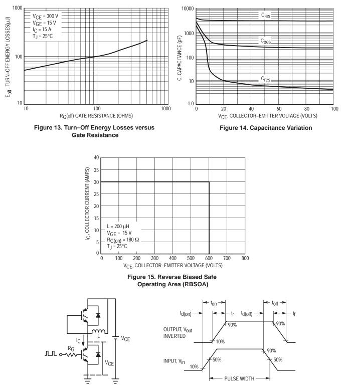
Figure 16. Inductive Switching Time Test Circuit and Timing Chart
