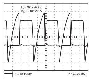
Figure 12–19. Steady State Operation (Vline = 230 V)
