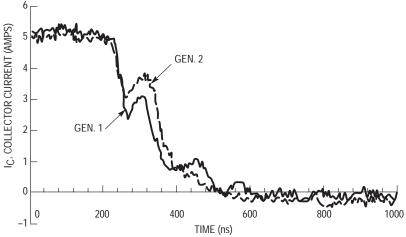
Figure 8–6. Tail Time Comparison of 600V Generation 1 and Generation 2 IGBT's in a 1 HP Motor Drive at 1750 RPM
