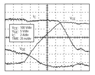
Figure 5–9. Turn–off at 120°C (V<sub>DD</sub> = 500 Vdc)
