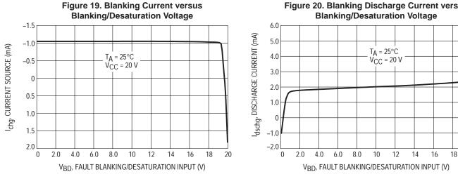
Figure 20. Blanking Discharge Current versus
