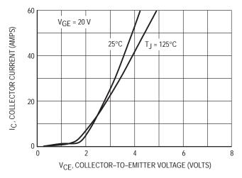
Figure 5–1. IGBT Output Characteristics
