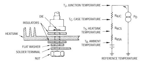
Figure A1. Basic Thermal Resistance Model Showing Thermal to Electrical Analogy for a Semiconductor
