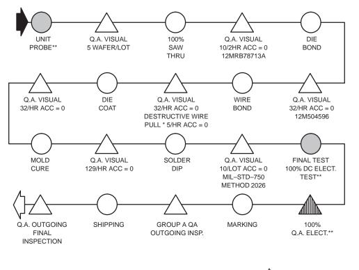
\*100% NON-DESTRUCTIVE WIRE PULL AFTER WIRE BOND \*\*100% DC ELECTRICAL TESTING ASSEMBLY PROCESS FLOW
