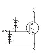
15 AMPERES N-CHANNEL IGBT VCE(on) = 1.8 V 380 VOLTS CLAMPED
