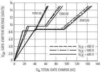
Figure 4. Gate–Emitter Voltage versus Total Gate Charge
