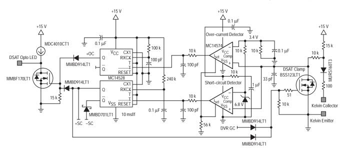
Figure 9–5. DSAT Overcurrent Detection and Shutdown Logic
