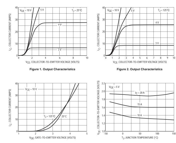
Figure 3. Transfer Characteristics
