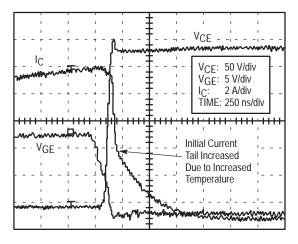
Figure 5–4b. Turn–off Waveforms at 120°C
