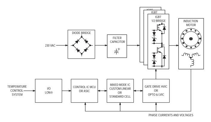
Figure 1–8. Typical Pulse–Width, Modulated, Variable–Speed Induction Motor Drives Are Where IGBT's Offer Performance Advantages
