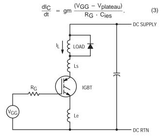
Figure 3–1. Clamped Inductive Load
