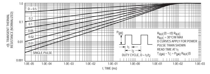
Figure 12. Typical Thermal Response
