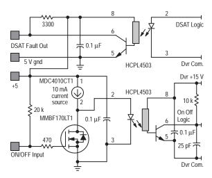
Figure 9–2. Optocoupler Interface Circuit for Input and Output Signals
