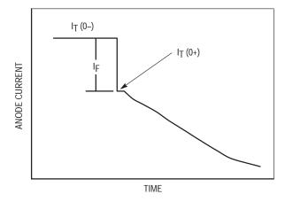
Figure 5–3. Anode Current During Turn–off
