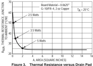
gure 3. Thermal Resistance versus Drain Pad Area for the D<sup>2</sup>PAK Package (Typical)
