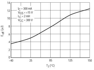
Figure 12–14. Switching Losses –E<sub>Off</sub>– as a Function of Temperature
