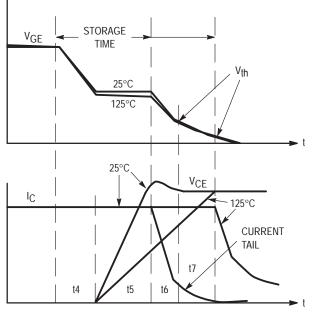
Figure 5–6. Turn–off Behavior of IGBT with Temperature Variations
