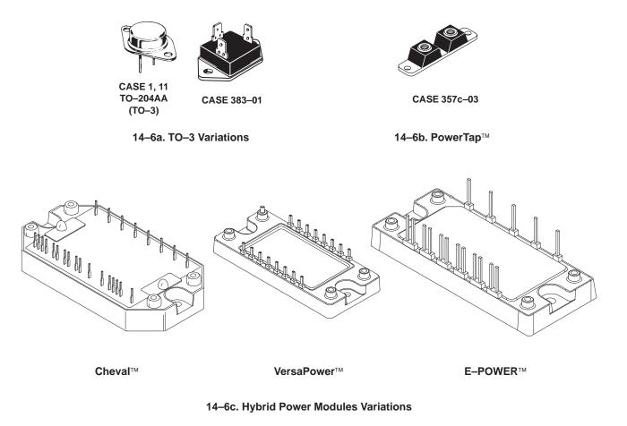
Figure 14–6. A Large Array of Parts Fit into the Flange–Mount Classification
