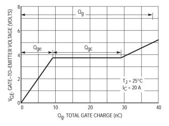
Figure 6. Gate-to-Emitter Voltage versus Total Charge
