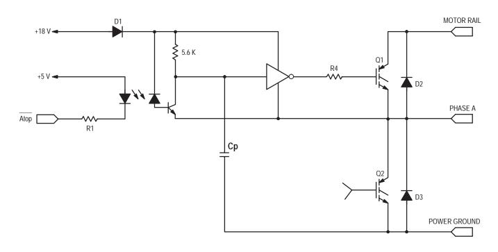
Figure 13–7. Parasitic Capacitance
