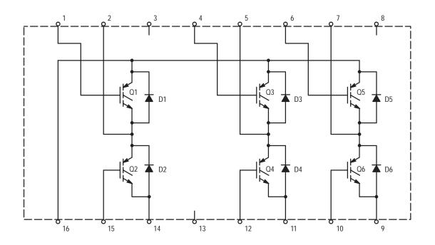
Figure 18. Schematic of Internal Circuit, Showing Package Pin–Out
