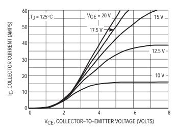
Figure 2. Output Characteristics
