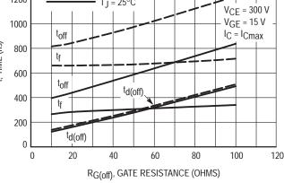
Figure 6. Inductive Switching Times versus **Gate Resistance**
