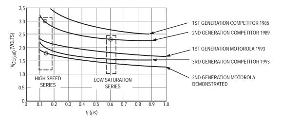
Figure 8–1. IGBT VCE(sat) Relation to Device Fall Time
