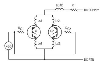
Figure 6–1. Paralleled IGBTs Used in Inductive Load
