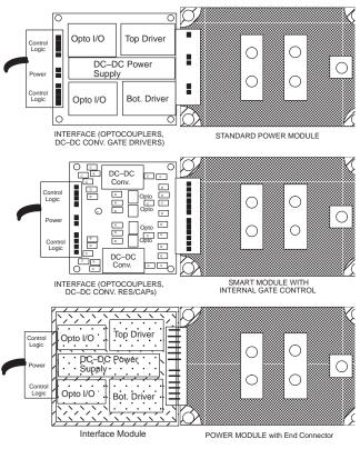
Figure 9–8. Power Module Circuit Attachment Options. Note how the smart module still requires an interface circuit board.
