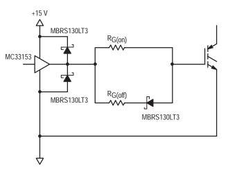
Figure 17. Recommended Gate Drive Circuit
