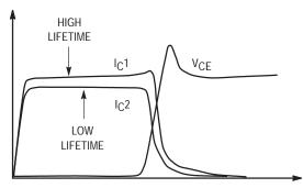
Figure 6–2. Paralleled Operation of IGBTs with Lifetime Variation
