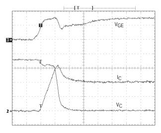
Figure 7–5b. IGBT Turn–On Test Waveforms for E–Series MGW21N60ED (100 ns/div) @ I<sub>C</sub> = 20 A,  $V_{CC}$  = 360 V,  $V_G/R_G$  = 15 V/20  $\Omega$ ,  $T_J$  = 125°C
