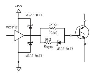
Figure 5. Recommended Gate Drive Circuit
