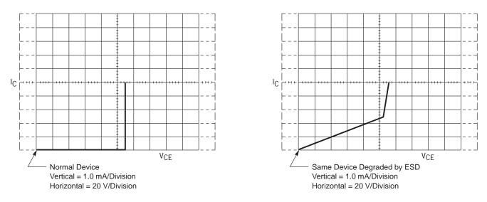
Figure 17–1. Curve Tracer Drawings of V<sub>CE</sub> versus I<sub>C</sub> of a Good Device (Left), and a Device in which the Gate was Damaged with ESD (Right). The Gate in this Device is Likely a Resistive Short.
