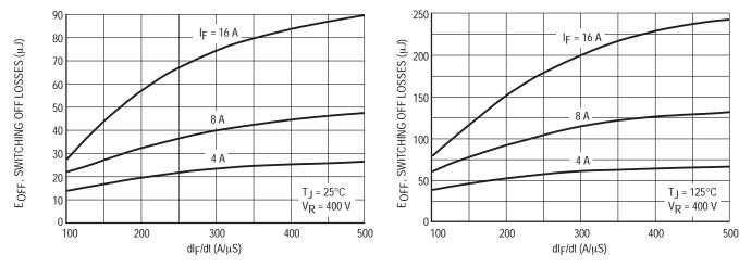
Figure 12. Typical Switching Off Losses
