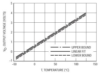
Figure 10–6. Linear Fit for Temperature Sense
