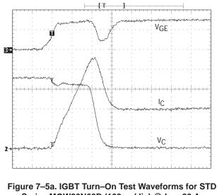
Series MGW20N60D (100 ns/div) @ I<sub>C</sub> = 20 A, V<sub>CC</sub> = 360 V, V<sub>G</sub>/R<sub>G</sub> = 15 V/20 Ω, T<sub>J</sub> = 125°C
