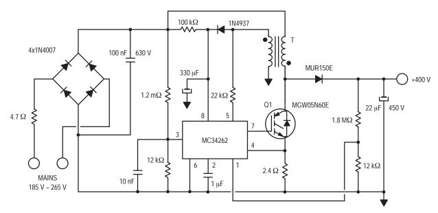
Figure 12–23. Basic Low Cost Power Factor Correction Circuit
