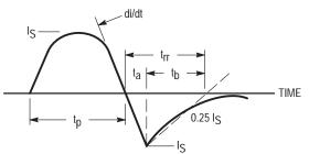
Figure 8. Diode Reverse Recovery Waveform
