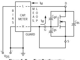
Figure 5. Cres Test Configuration
