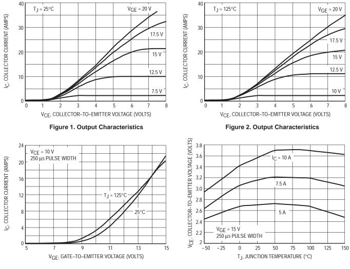
Figure 3. Transfer Characteristics
