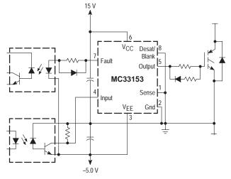
When used in a dual supply application as in Figure 35, the Kelvin Ground should be connected to the emitter of the IGBT. If the protection features are not used, then both the Fault Blanking/Desaturation and the Current Sense Inputs should be connected to Ground. The input optoisolator should always be referenced to  $V_{FF}$ .
