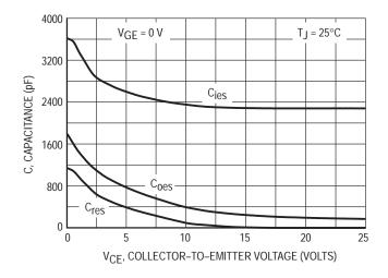
Figure 3–4. IGBT Capacitance Curves
