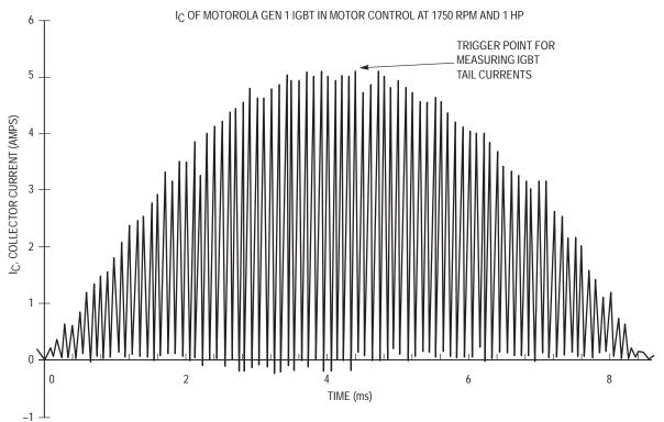
Figure 8–4. IGBT Collector Current
