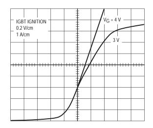
Figure 11–3. IGBT Saturation Voltage
