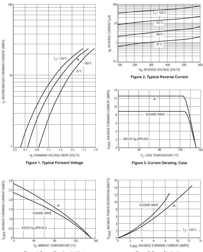
Figure 4. Current Derating, Ambient
