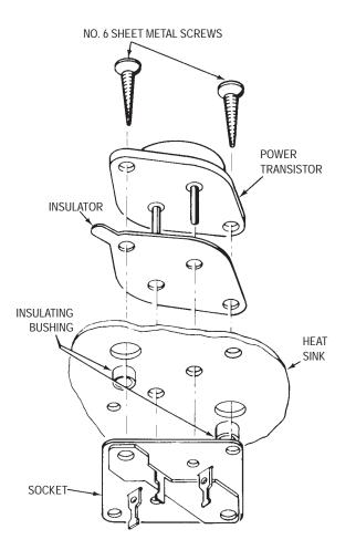
Figure 14–7. Hardware Used for a TO–204AA (TO–3) Flange Mount Part
