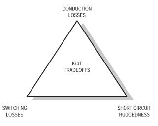
Figure 7–1. IGBT Tradeoff Triangle
