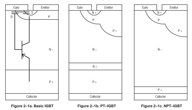
Figure 2-1. Insulated Gate Bipolar Transistors Cross Sections (not to scale)
