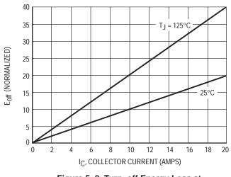
Figure 5–2. Turn–off Energy Loss at Different Temperatures
