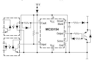
When using sense IGBTs or a sense resistor, as shown in Figure 33, the sense voltage is applied to the current sense input. The sense trip voltages are referenced to the Kelvin Gnd pin. The sense voltage is very small, typically about 65 mV, and sensitive to noise.
