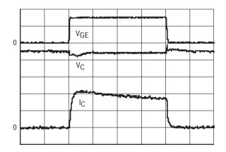
Figure 7–6b. IGBT Short Circuit Test Waveforms @  $125^{\circ}$ C for E–Series MGW21N60ED (250 ns/div) Scales: IC – 50 A/div, V<sub>CC</sub> – 100 V/div, V<sub>G</sub> – 10 V/div
