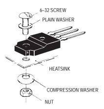
14–12b. Screw–Mounted Isolated Package
