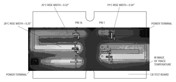
Figure 10–7. Two Sided, 3 oz. Copper at 25 A VersaPower™ Package Pin Footprint
