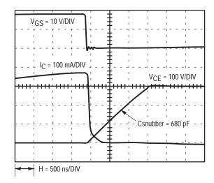
Figure 12–20. Switching Losses in the Steady State
