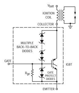
Figure 11–2. IGBT with Integral Collector–Gate and Gate–Emitter Clamps in an Ignition Circuit
