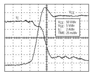
Figure 5–7. Turn–off at 25°C (V<sub>DD</sub> = 300 Vdc)
