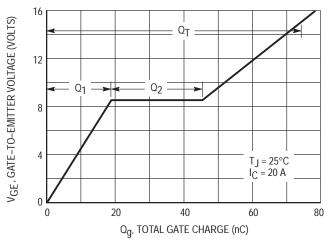
Figure 3–5. Gate Charge Transfer Curve
