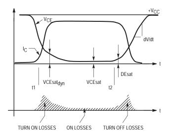
Figure 12–17. Switching Time and Loss Definitions
