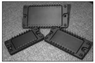
Figure 10–4. 16, 20 and 24 Pin VersaPower™ Packages
