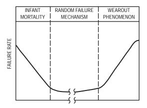
Figure 16–3. Failure Rate of Semiconductor
