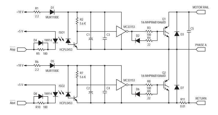
Figure 13–2. Robust N–Channel IGBT Power Stage
