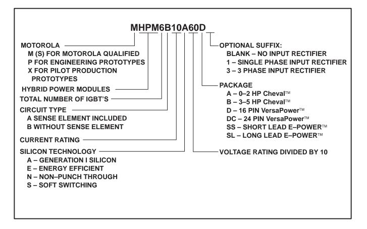
Figure 2. Motorola Module Part Numbering System
