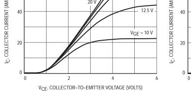
**Figure 1. Output Characteristics**
