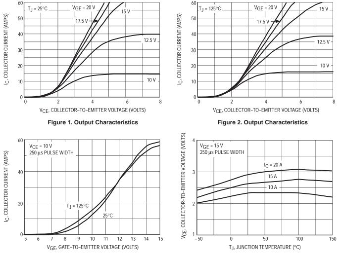
Figure 3. Transfer Characteristics
