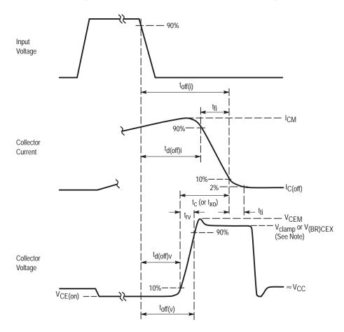
NOTE: V<sub>clamp</sub> (in a clamped inductive–load switching circuit) or V<sub>(BR)CEX</sub> (in an unclamped circuit) is the peak off–state voltage excluding spikes.
