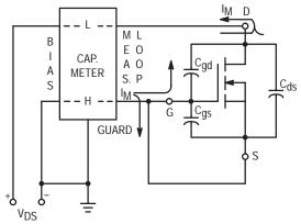
Figure 4. Coes Test Configuration
