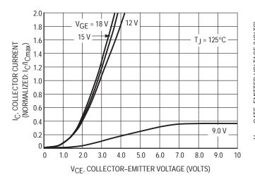
Figure 3. Forward Characteristics, T<sub>J</sub> = 125°C
