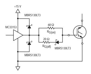
Figure 5. Recommended Gate Drive Circuit
