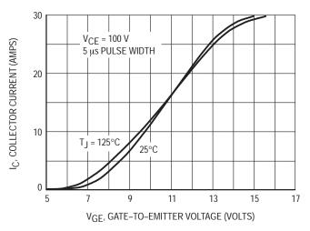
Figure 3. Transfer Characteristics
