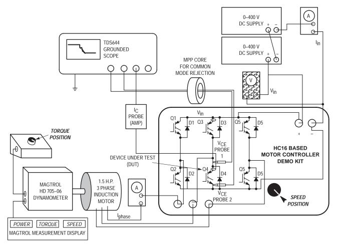
Figure 8–2. 1 HP Variable Speed Motor Drive Test Bed
