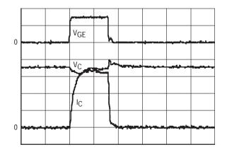
Figure 7–6a. IGBT Short Circuit Test Waveforms @  $125^{\circ}$ C for STD Series MGW20N60D (250 ns/div) Scales: IC – 50 A/div, V<sub>CC</sub> – 100 V/div, V<sub>G</sub> – 10 V/div
