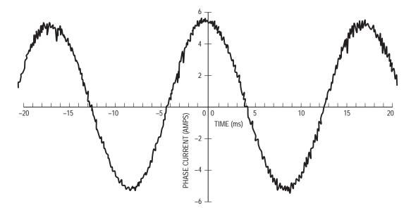
Figure 8–3. Motor Phase Current
