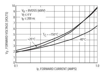
Figure 12–9. PowerLux™ IGBT Diode Characteristics
