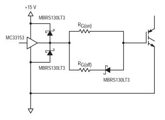
Figure 17. Recommended Gate Drive Circuit
