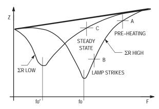
Figure 12–3. RLC Series Resonant Network Behavior
