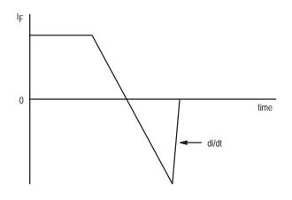
Figure 13–5. Drain–Source Diode Snap
