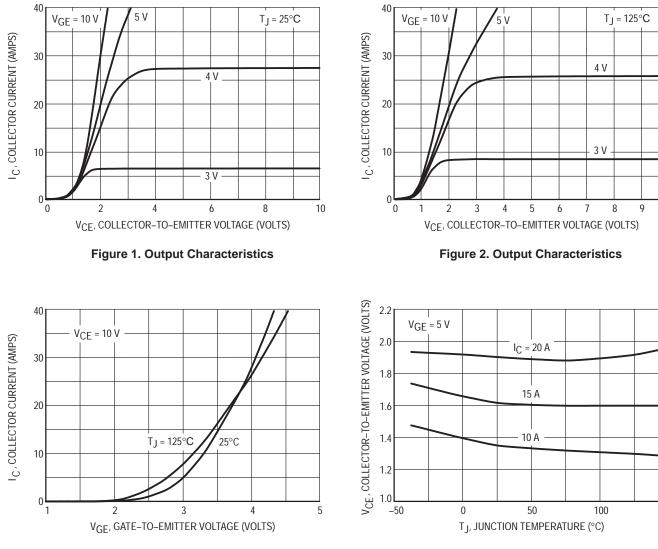
Figure 3. Transfer Characteristics
