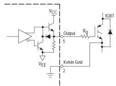
An optimized gate drive output stage is shown in Figure 31. This circuit allows turn-on and turn-off to be optimized separately.
