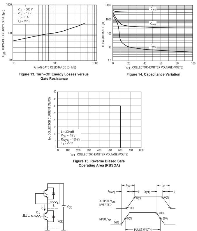
Figure 16. Inductive Switching Time Test Circuit and Timing Chart
