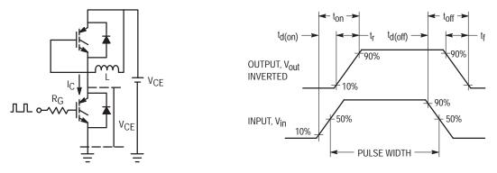
Figure 18. Inductive Switching Time Test Circuit and Timing Chart
