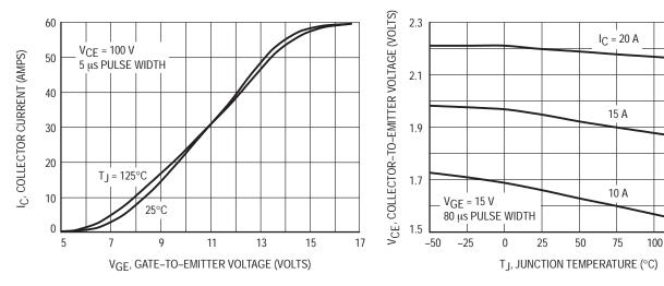
Figure 3. Transfer Characteristics
