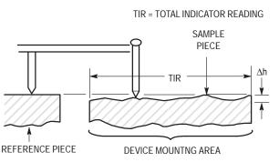
Figure 14–2. Surface Flatness Measurement
