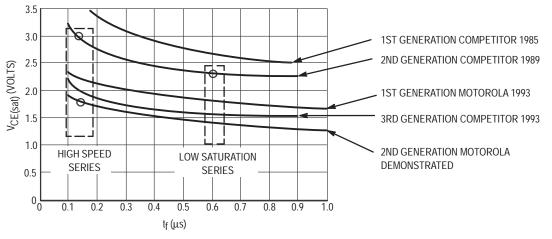
Figure 1–2. Advanced Features Offered by the Latest Motorola IGBT Technologies for Forward Voltage Drop (V<sub>CE(sat)</sub>) and Fall Time (t<sub>f</sub>)
