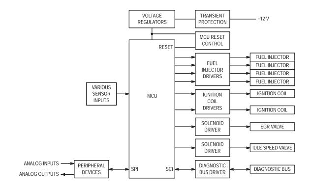
Figure 11–1. MCU–Controlled Direct Fire Ignition System
