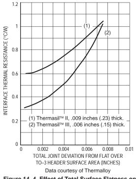
Figure 14–4. Effect of Total Surface Flatness on Interface Resistance Using Silicon Rubber Insulators
