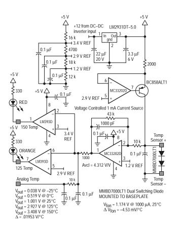
Figure 9–6. Temperature Detector Circuit uses a Dual Diode Sensor
