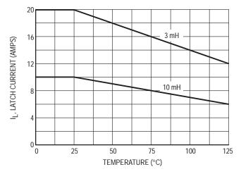
Figure 7. Latch Current versus Temperature
