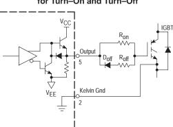
Figure 27. Using Separate Resistors for Turn–On and Turn–Off
