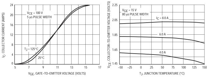
Figure 3. Transfer Characteristics
