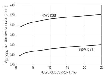
Figure 11–6. Clamped IGBT Voltage Variation With Current
