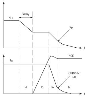
Figure 3–6. Idealized Turn–off Switching for IGBT
