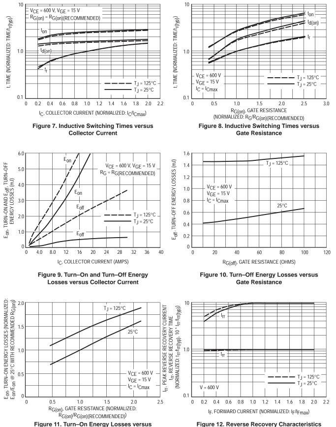
Figure 11. Turn–On Energy Losses versus Gate Resistance
