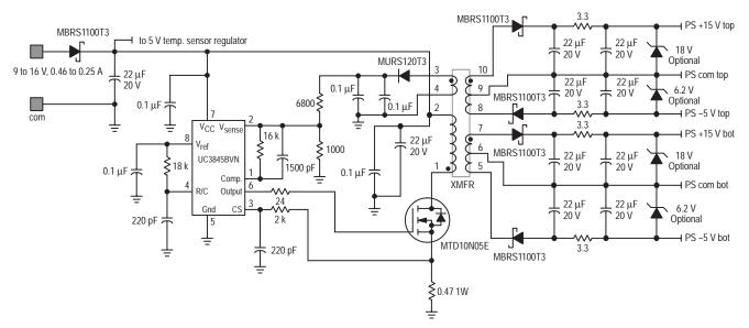
Figure 9–7. DC–DC Power Supply for 1/2 Bridge Control Circuit
