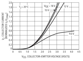
Figure 2. Forward Characteristics, T<sub>J</sub> = 25°C
