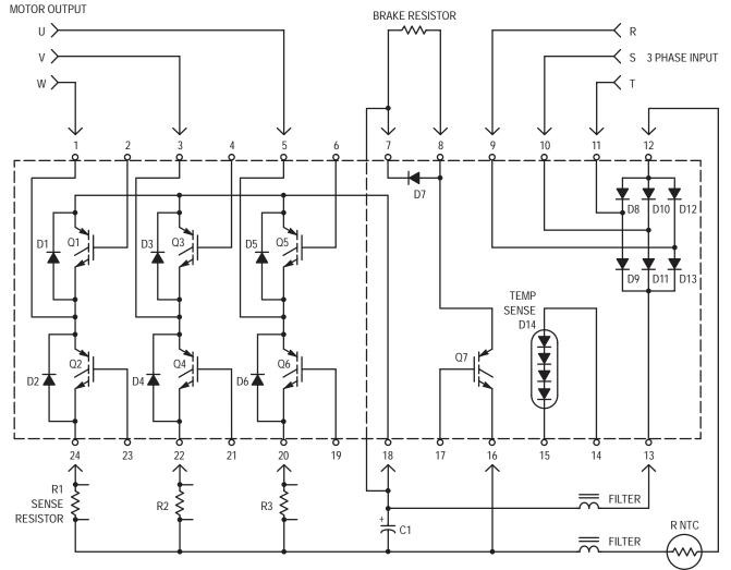
Figure 10–3. 24 Pin VersaPower™ IPS with Brake & Temp Sense
