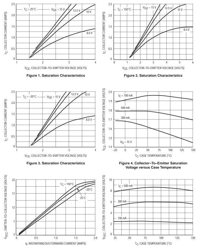
Figure 6. Diode Forward Voltage versus Case Temperature
