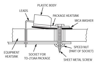
Figure 14–1. Extreme Case of Improperly Mounting a Semiconductor (Distortion Exaggerated)
