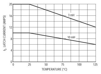
Figure 7. Latch Current versus Temperature
