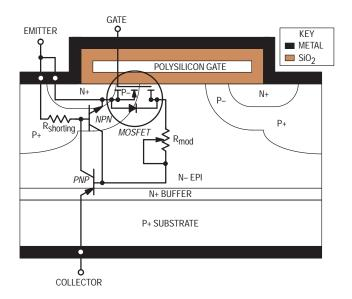
Figure 1–3a. Cross Section and Equivalent Schematic of an Insulated Gate Bipolar Transistor (IGBT) Cell
