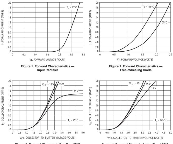
Figure 3. Forward Characteristics, T<sub>J</sub> = 25°C
