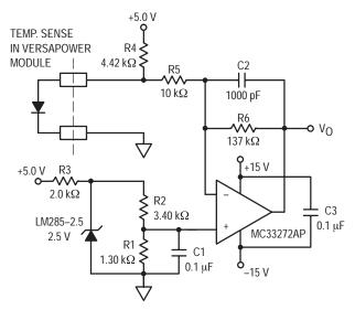
Figure 10–5. Temperature Sense Circuit
