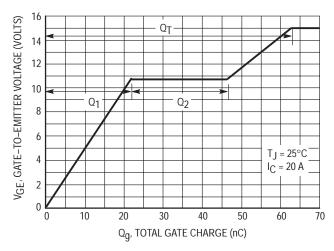
Figure 6. Gate-to-Emitter Voltage versus Total Charge
