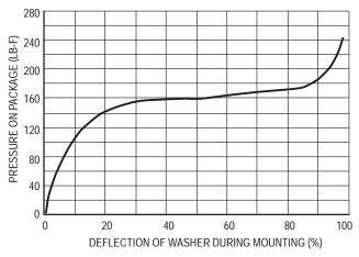
Figure 14–5. Characteristics of the Conical Compression Washers Designed for Use with Plastic Body Mounted Semiconductors
