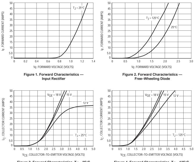
Figure 3. Forward Characteristics, T<sub>J</sub> = 25°C
