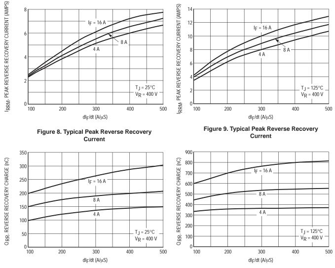
Figure 10. Typical Reverse Recovery Charge
