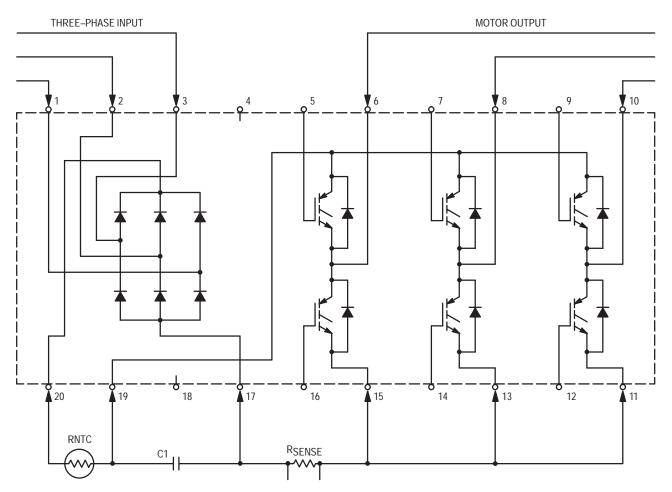
Figure 10–2. 20 Pin VersaPower<sup>™</sup> with a 3 Phase Input Bridge and 6–Pack Output
