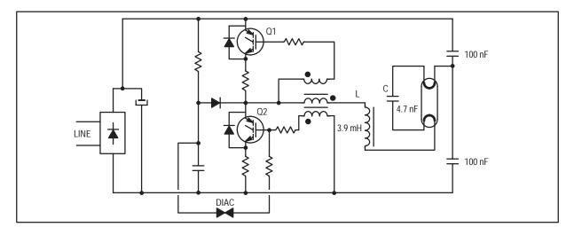
Figure 12–1. Basic Self Oscillant CFL
