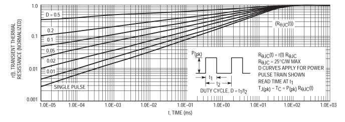
Figure 12. Typical Thermal Response
