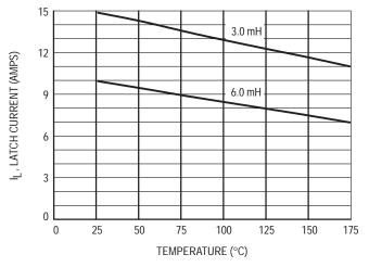
Figure 11. Latch Current versus Temperature
