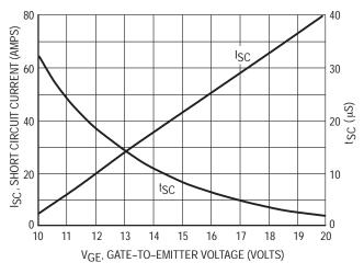
Figure 4–3. Short Circuit Response of IGBT
