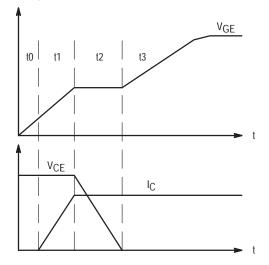
Figure 3–2. Idealized Turn-on Switching of IGBT
