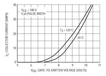
Figure 3–3. Gate–Emitter Voltage Due to Temperature Variation
